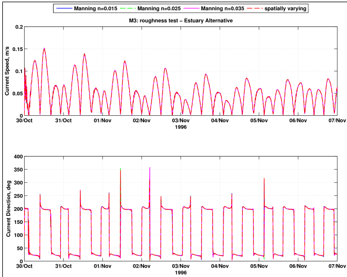
Figure 4-37 Modeled Current Velocity at Station M3 with Varying Manning for Estuary Alternative
