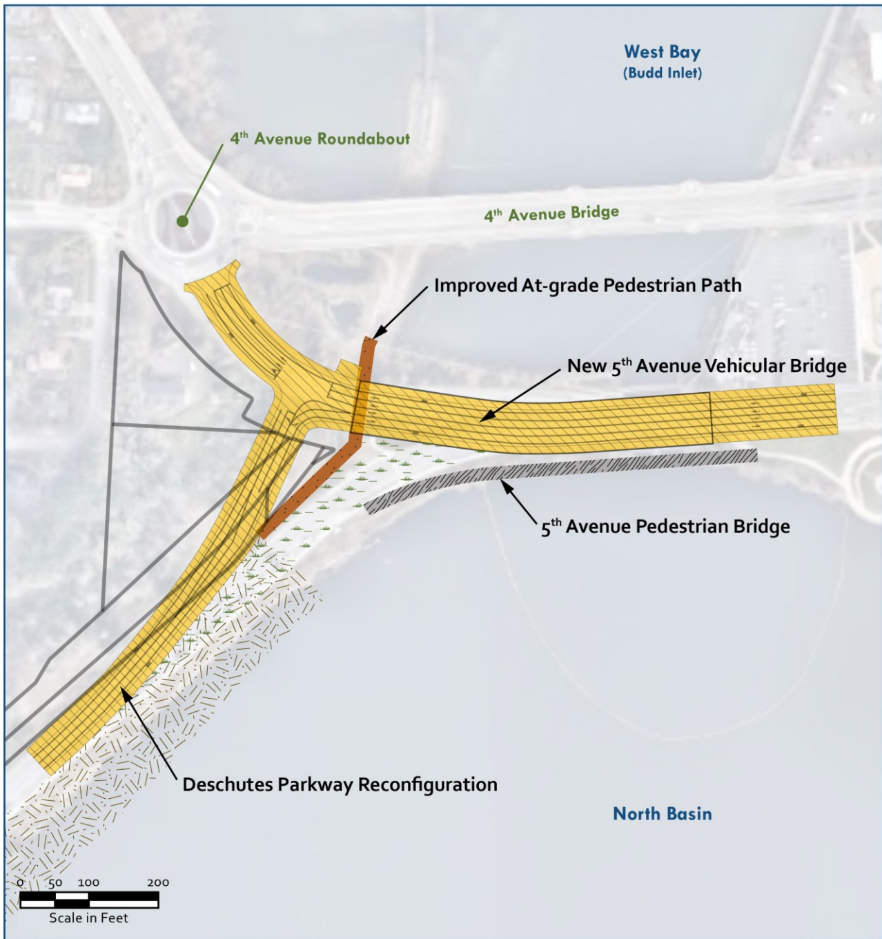
Figure 2.4.4 Deschutes Parkway Realignment & New 5th Avenue Bridge
